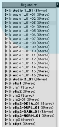
Figure 3-10: Audio files created by recording into an audio track show up in the Regions list.
